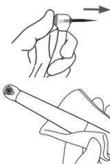
Remove the bur from the handpiece, turn on the water supply switch on the dental treatment unit, then run the motor (idle running) for 20 seconds.
