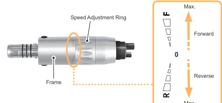
Hold the frame part and rotate the speed adjustment ring to switch the rotation direction and change the speed.
