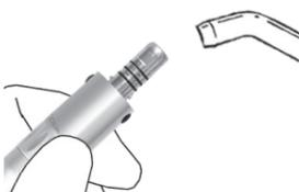
After cleaning, use the syringe or an air blow gun to blow out any moisture remaining inside the motor to dry it out.
