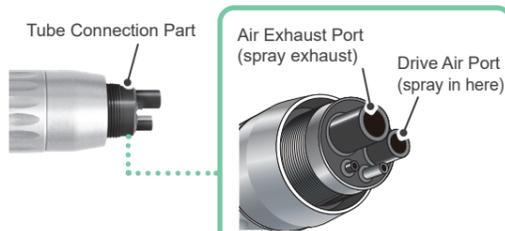
Insert the spray nozzle into the drive air port.
