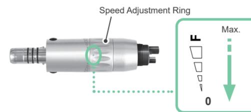
Turn the speed adjustment ring and set it from F (maximum position) to 0.
