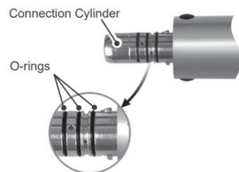
Remove the O-rings with tweezers or another such tool and install the replacements.
