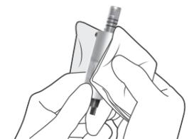
Wipe the motor with a piece of gauze or microfiber cloth (e.g., Toraysee for CE - Medical Equipment and Instruments Maintenance Cloth) that has been dampened with mikrozid AF liquid, FD322, or rubbing alcohol to remove visible contaminants.
