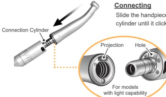
\* For handpiece models with light capability, give the handpiece a slight press toward the motor and turn the handpiece until the projection on it lines up with the notch in the motor. You can hear an audible click when the projection and notch line up.
