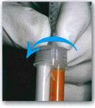
This photo shows the VPS material just at the mixing tip without entering it. The tab has been rotated 90° to the position above "\Lambda" (Chevron).
