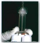
The cartridge whether 25, 50, or 75ml is firmly butted into the barrels so that there is a tight fit at the base of the syringe.
